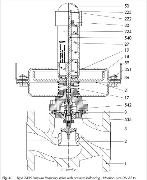
Fig. 4: Type 2405 Pressure Reducing Valve with pressure balancing · Nominal size DN 32 to 50 · Set points 0.005 to 0.060 bar · Flow-to-open (two-step control mode)
