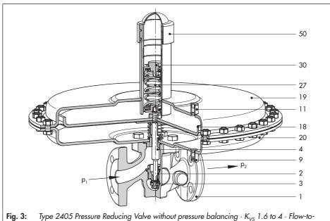
**Fig. 3:** Type 2405 Pressure Reducing Valve without pressure balancing  $\cdot$  K<sub>VS</sub> 1.6 to  $4 \cdot$  Flow-to open
