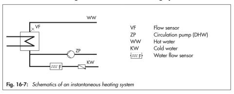
Without flow rate sensor or flow switch, the control of the required DHW temperature at the flow sensor VF is only active during times-of-use of the circulation pump ZP. The water flow sensor or flow switch allows the controller to recognize when DHW tapping starts and stops. Control of the required DHW temperature can made to be active only during DHW tapping by deleting all times-of-use of the circulation pump.
