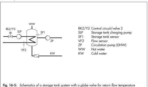
Globe valve and flow sensor VF2 are used exclusively for return flow temperature limitation in the schematics shown above. The pre-control circuit provides at least the same flow temperature as in the standard schematic version which is calculated from 'DHW temperature set point' + 'Charging temperature boost' + 'Boost set point (pre-control circuit)'.
