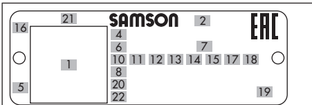
Fig. 2-2: Inscriptions on the valve nameplate
