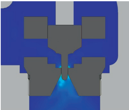
Fig. 4: CFD velocity profile for ZT-1-II in an angle valve
