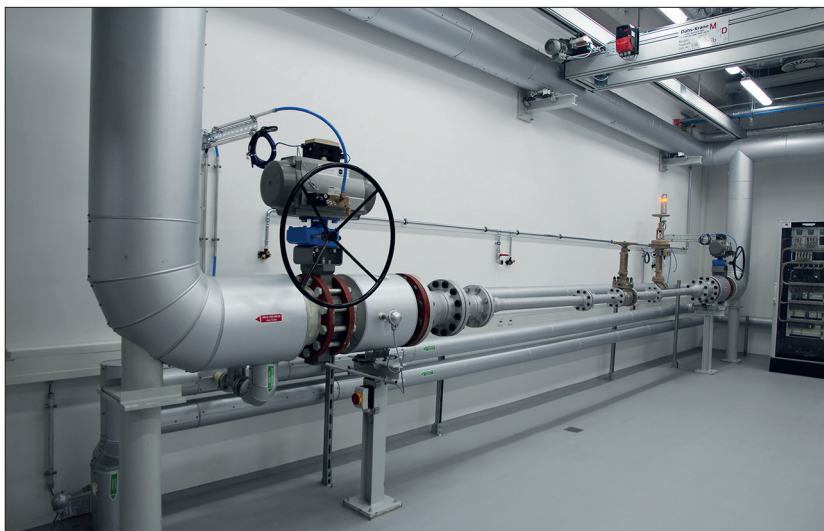
In this Flow Lab, the functions of non-powered controllers are tested as separate components in simulated district heating networks: valve sizes DN 15 to 300 for steam at a temperature of 230 °C to 13 bar pressure and a flow rate of 5,000 kg/h
